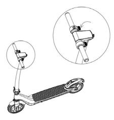
CRUISE CONTROL: The scooter maintains your selected speed when the THROTTLE LEVER is held in the same position for 5 seconds. An audible "BEEP" will be heard when CRUISE CONTROL engages. To Turn off CRUISE CONTROL mode, press the BRAKE LEVER located on the left side of the handlebar.
