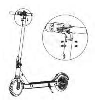
Fix the handlebars with the 4 screws provided. Use the M4 Hex Key to attach the handlebars to your scooter. Make sure it is secure and the handlebars are stable before using your scooter.
